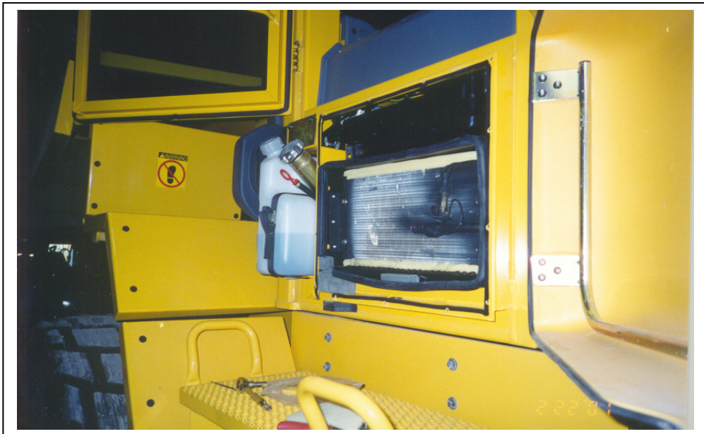
End view of evaporator assembly in place.
