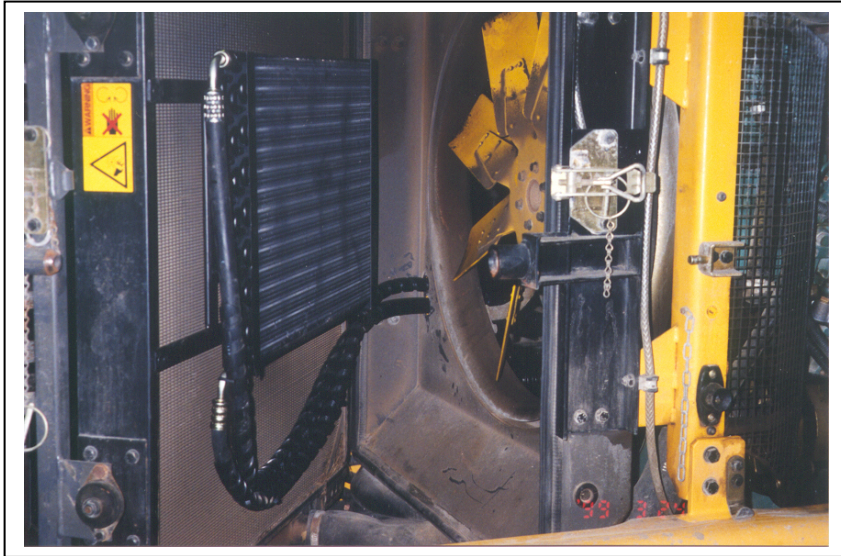
Condenser view showing the mounting set-up with hoses into engine compartment.
